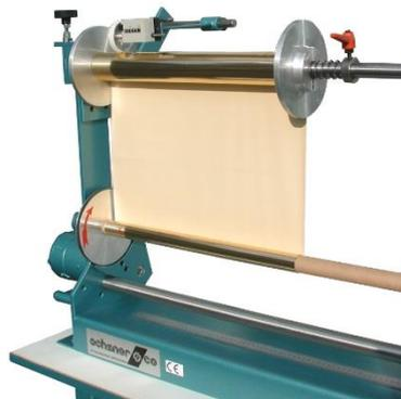
RG machine with option winding unit and linear measure unit
