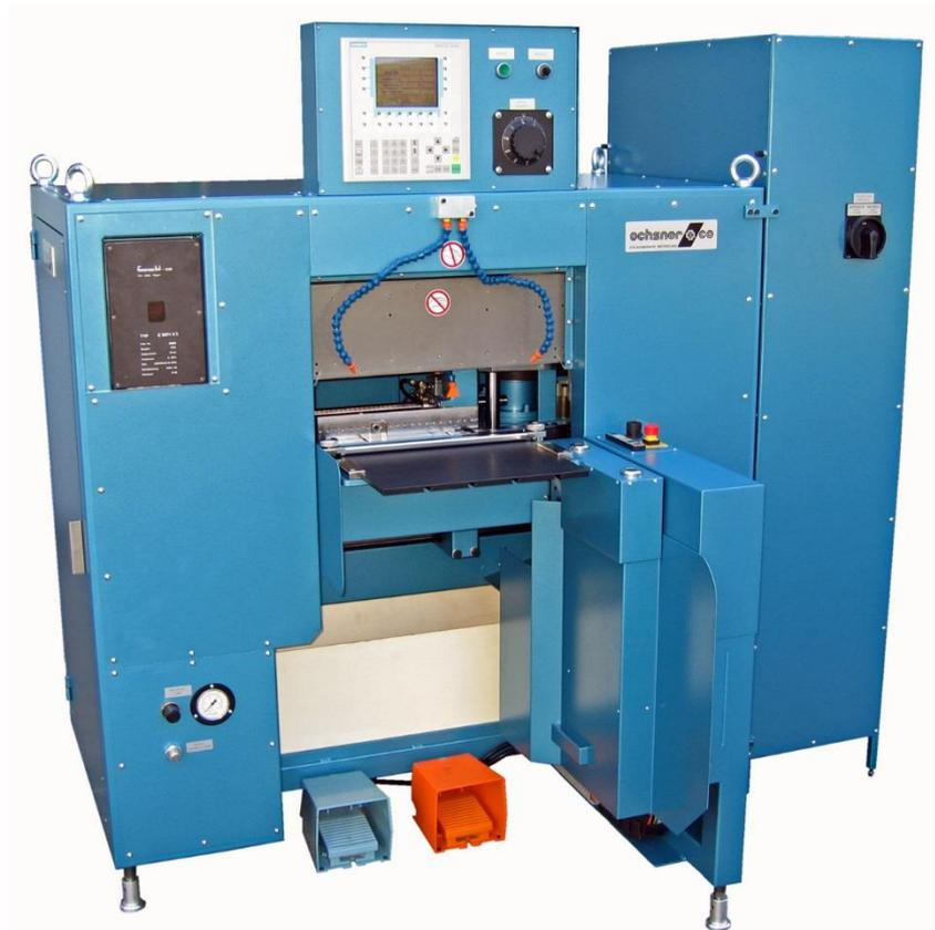
With this machine you can cut many different index styles. All machine details are displayed on a screen. With a hand wheel you can program the needed position for every axle without a computer (teaching). The working table with the book is fix but the knife moves from cut to cut.
