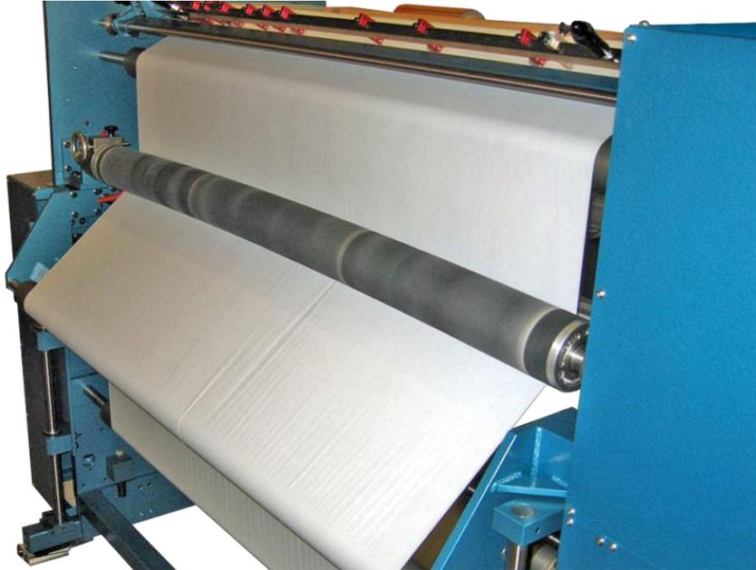
The function of this spread roller is to flatten the web before rewinding. As you can see on the picture, there are no more wrinkles after the spread roller.
