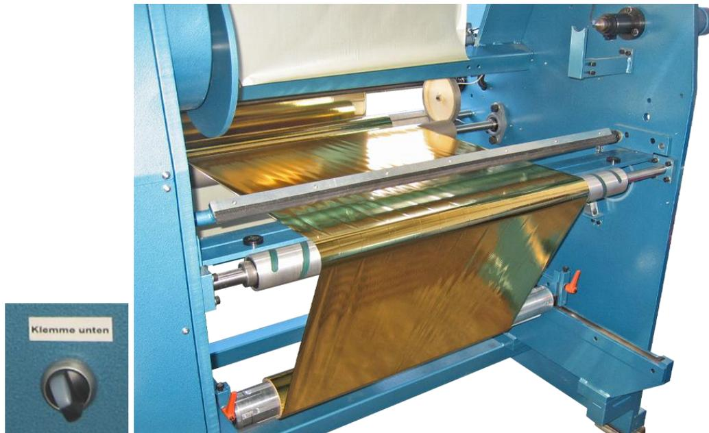
The splicing table is helpful when the Jumbo needs to be change. The foil will stay under tension in the machine and the new foil can be spliced to the existing foil. Another useful function is to make a gap between the foil and put a self-adhesive tape on the gap. After running this web through the machine and blades, you have the foil end automatically taped to the roll end. A time-consuming applying of stickers or labels at the end will be eliminated.
